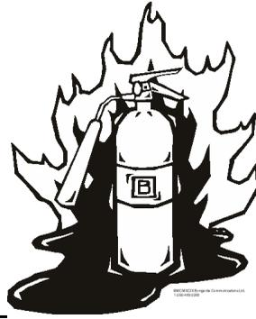
Fire extinguishers are tested by independent testing laboratories and are labeled for the type of fire they are intended to extinguish. There are four classes of fires. All fire extinguishers are labeled, using standard symbols, for the classes of fires they can be used to fight. A red slash through any of the symbols tells you the extinguisher cannot be used on that class of fire.
